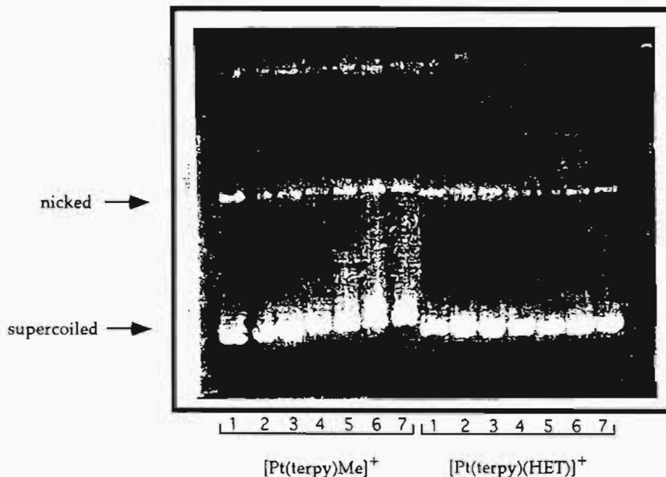
**Figure 7.** Gel electrophoresis in 1.2% agarose gels of pUC 19 DNA incubated with different amounts of  $[\text{Pt}(\text{terpy})\text{Me}]\text{Cl}$  and  $[\text{Pt}(\text{terpy})(\text{HET})](\text{NO}_3)$  in TBE running buffer at 25 °C for 30 min. Lanes: (1)  $r_f = 0$ ; (2)  $r_f = 0.017$ ; (3)  $r_f = 0.035$ ; (4)  $r_f = 0.052$ ; (5)  $r_f = 0.070$ ; (6)  $r_f = 0.078$ ; (7)  $r_f = 0.087$ .
