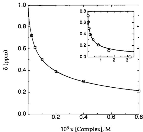
**Figure 3.** Concentration dependence of  $^1\text{H}$  NMR chemical shift for the methyl group of  $[\text{Pt}(\text{terpy})\text{Me}]\text{Cl}$  in  $\text{D}_2\text{O}$  at 298 K (see text for details).
