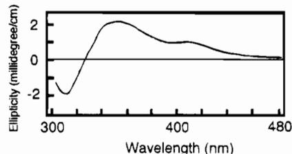
**Figure 6.** CD spectra of [Pt(terpy)Me]Cl in the presence of *ct*-DNA. Experimental conditions: [complex] = 0.05 mM; [DNA] = 1 mM in buffer A at 298 K.
